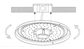
4). Insert wire into junction box ,then rotate panel when justify the screws at the screw holes.
